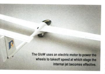
op would be great if the jet engine could be used to actually launch the glider but so far this has proved impractical as the static thrust of these jet engines is too low to launch a glider from a standing start. This problem of how to get things going has been solved by ProAirsport's innovative jet-powered SSDR self-launcher.
